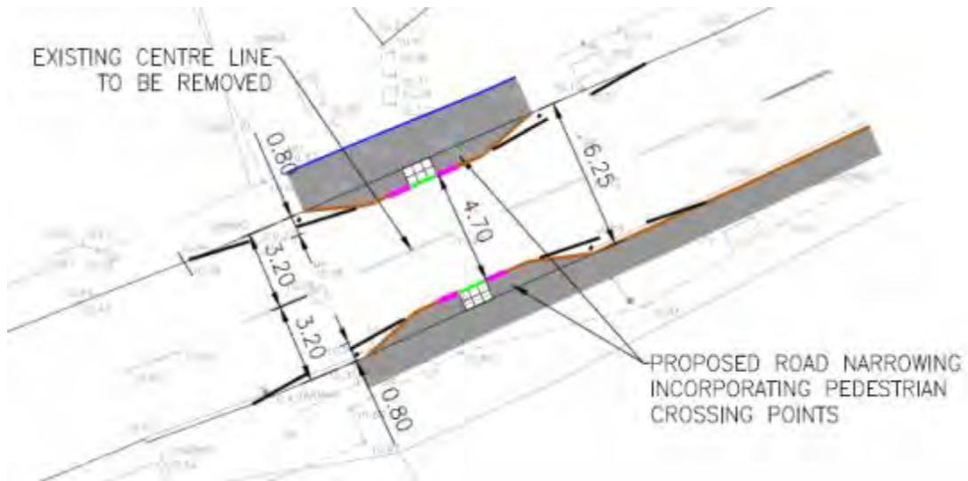
Photo 4: Example of road narrowing and pedestrian crossing point (Ringmer)
